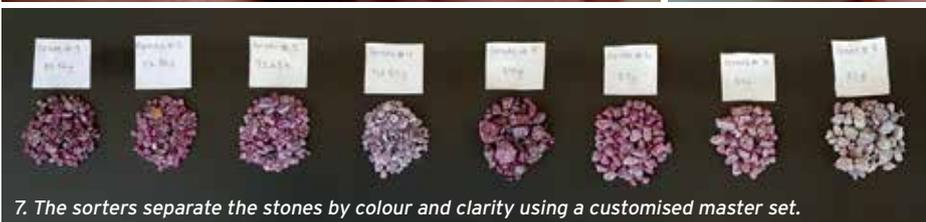
7. The sorters separate the stones by colour and clarity using a customised master set.
